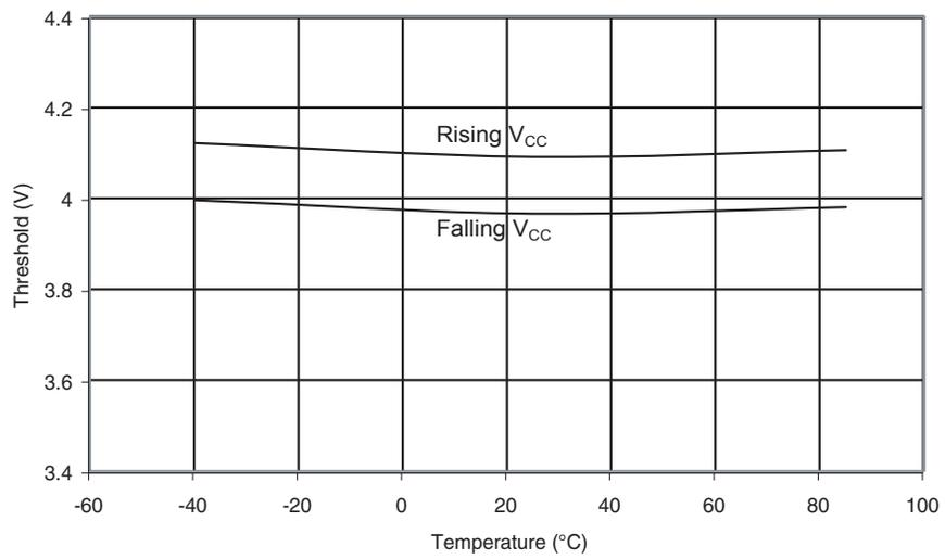
Figure 190. BOD Threshold vs. Temperature (BODLEVEL is 2.7V)
