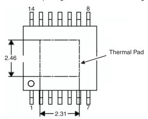
Figure 14. Thermal Pad Dimensions
