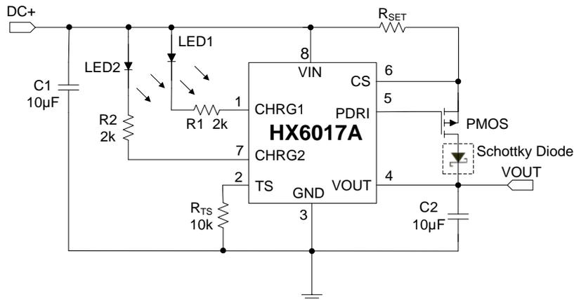
\*The charge current  $I_{O(REG)} = V_{CS}/R_{SET}$  ( $V_{CS}$  is usually 200mV). Note that OFF indicates the open-drain transistor is turned off.
