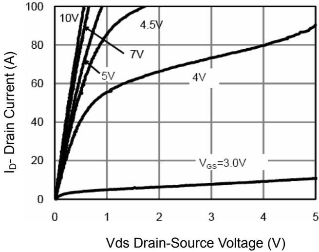
**Figure 1 Output Characteristics**
