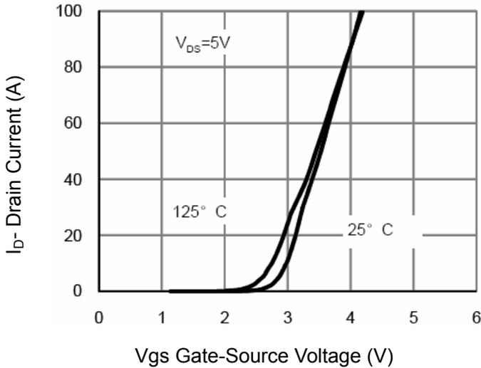
**Figure 2 Transfer Characteristics**
